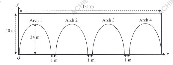
A civil engineer is designing a bridge which is 131 metres long, 40 metres high and is to have four identical parabolic arches along its length. Each arch is 34 metres high and there is one metre between bases of each adjacent pair of arches as shown in the diagram. A set of axes is placed with the origin at the left- hand end of the base of the first arch.
